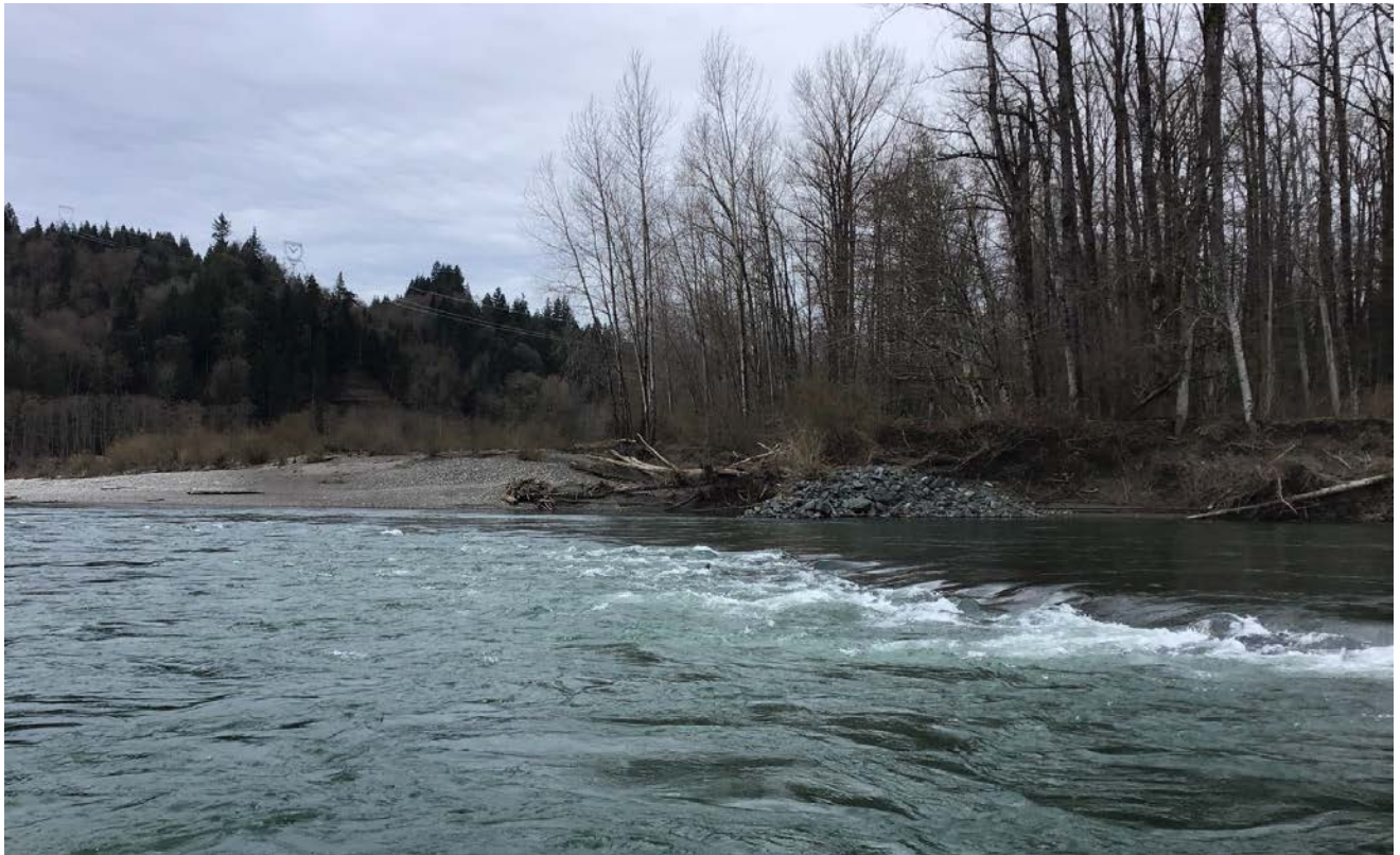
Figure 3. Skiyou rock, view from center of the channel towards the right bank. Flow direction is from right to left of photo. Note that the rock is overtopped at the time of survey during a flow of approximately 13,900 cfs. Bank rock is visible in the background (March 10, 2020).
